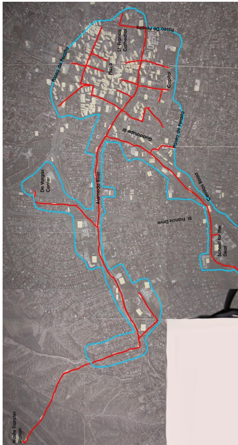
Figure 1: Target area and proposed path of the network of pipes – heat demand inquiry Santa Fe
